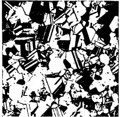
FIGURE 392. Metallographic structures of annealed cartridge brass (70% Cu — 30% Zn), grain size 0.050–0.055 mm. Etched with \text{NH}_4\text{OH} + \text{H}_2\text{O}_2 . \times 75 . (Left) Light etch. (Right) Contrast etch.
